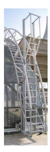
Normally ladders are used to climb from one level to another and real work is not recommended from them. However the Rostek traversing ladders are designed for work. Light construction work, repairs and maintenance tasks like window cleaning are typical tasks performed from the Rostek ladders.
