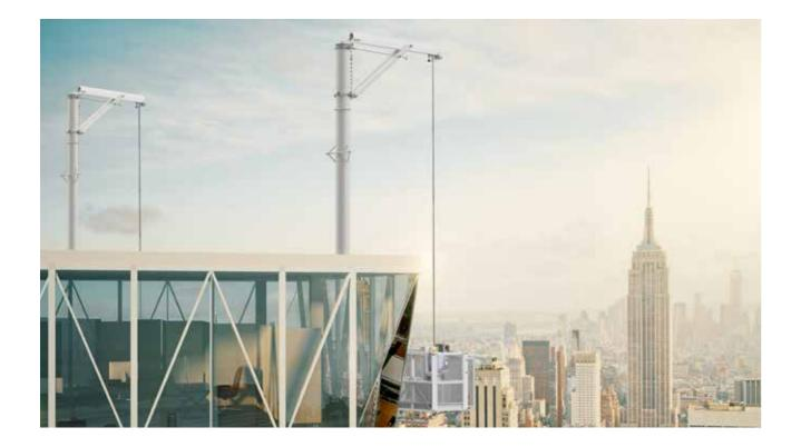
A davit looks like a simple, small crane used for suspending platforms. A davit system consists of two main parts: the portable davit and the base plate or pedestal. The davit is the visual part and the base is plate mounted to the roof to which the davit is attached to.
