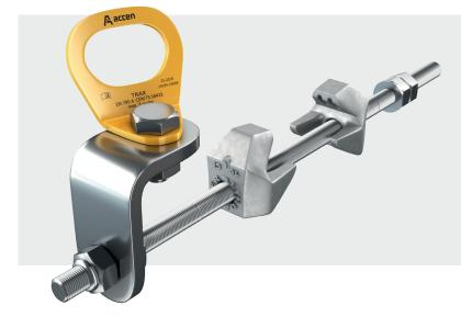
Anchoring point TRAX CLAMP is an anchoring device mounted to steel T-sections (T-beam and I-beam), intended for attaching devices of individual protection to prevent from falling from a height for maximum three persons at the same time. It comes in two installation versions - TRAX CLAMP and TRAX CLAMP XL.
