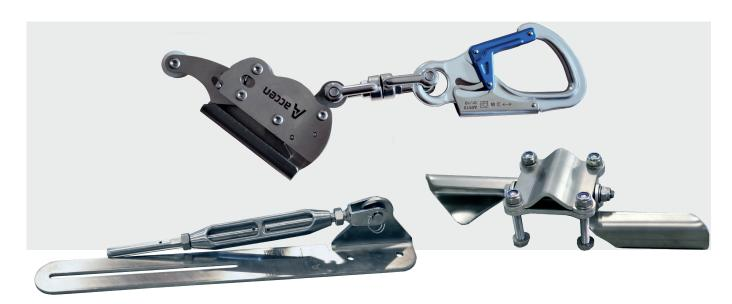
Vertic Line is a vertical fall protection system used on ladders and vertical passageways. The system is attached to the ladder rungs by means of special brackets. The upper point is equipped with a special shock absorber that suppresses the forces generated when the worker falls off. The maximum user weight is 150 kg.
