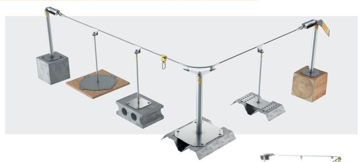
The Accen Line I is a horizontally installed 8 mm diameter steel wire rope that acts as a guide to which the user is attached.
